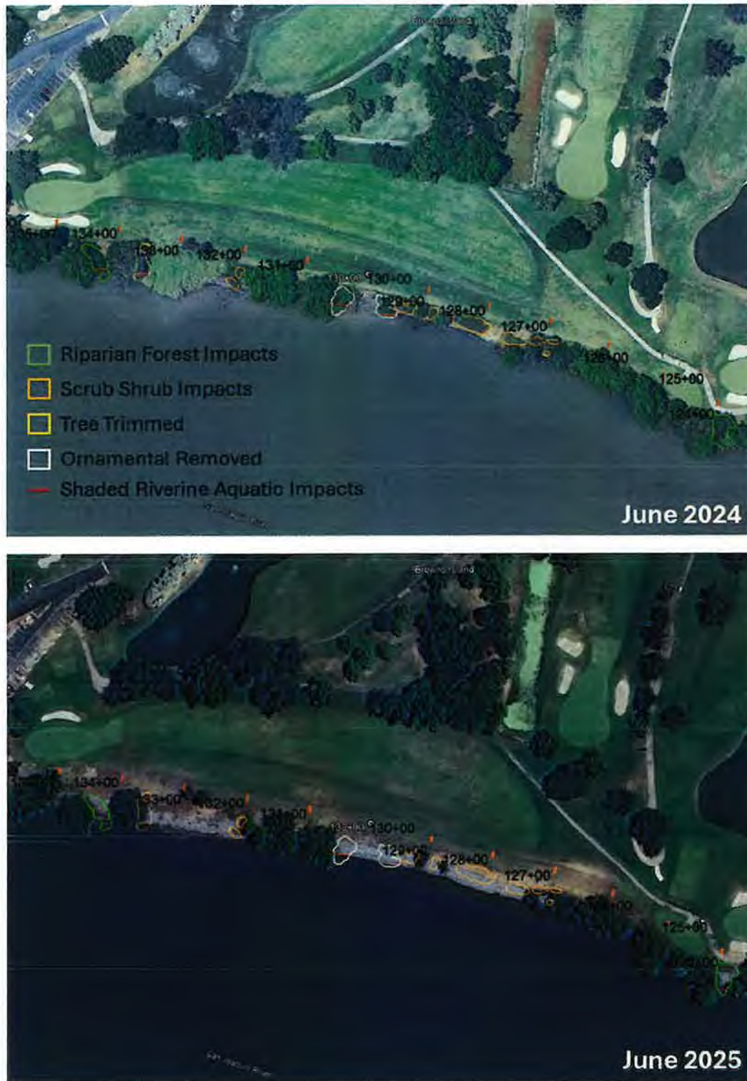
Figure 1. Before and after impacts on the Smith Tract waterside levee.
